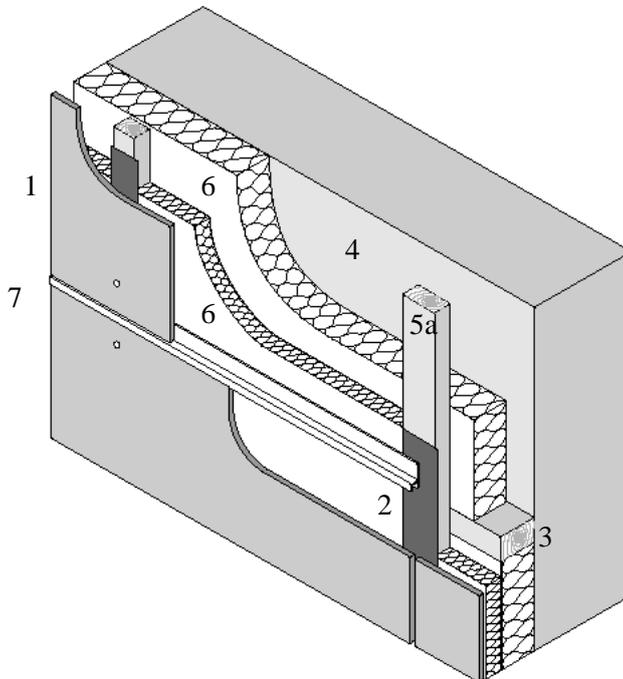
Figure 2. Ventilated intended use on vertical metal subframe
